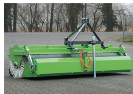
bema 20 AgrarLine: main brush Ø 520 mm (PPN), working width 2300 mm, rope pull, tractor rear
